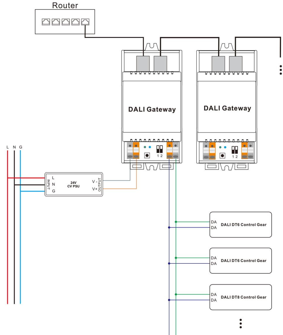
**Note:** When built-in DALI Bus PS is enabled, a DALI gateway can supports up to 64 control gears.
