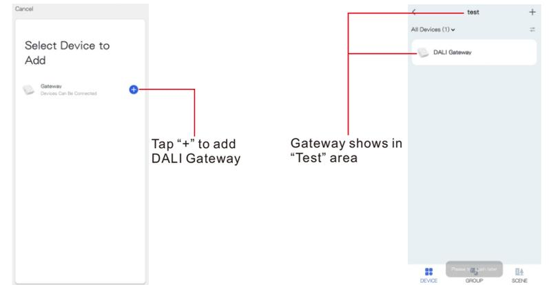
**Step 3:** The gateway was added successfully, then select the gateway to configure the following DALI devices.
