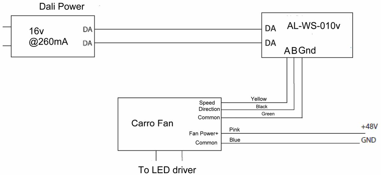
Connecting a AL-WS-Carro motor control to a Ceiling Fan
