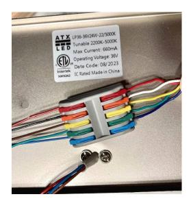
Connect the 4 wires from the Signature Fixture to the AL-WS-DR2 you can then adjust from 2200K to 5000K
