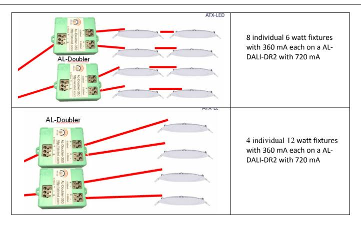
In addition, overcurrent protection is built in. In case a LED fails, or if the 2 loads are different wattages – the other string will be limited to 380ma max. If currents in excess are supplied by the driver – the working LED will operate at 10 ma – 400 milliwatts in most LED's. This provides enough light for people to navigate a room at night or to identify a bad LED.
