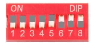
8 DIP switches on the side control the starting addresses for DALI groups in the DMX512 universe. Only even addresses can be set, from 2 thru 480... DALI drivers area assigned to groups via DALI master like the Euchips DALI-100, the AL-DALI-PI or set manually in the AL-WS-010v. The above example sets a base of 448.
