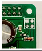
The device can be powered from the Raspberry Pi 3B+ PoE pins.
